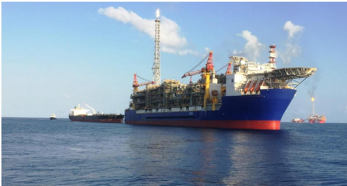
Shipping of condensate from the Floating Production, Storage and Offloading (FPSO) facility “Ichthys Venturer” and the Central Processing Facility “Ichthys Explorer” in the background (far right)
