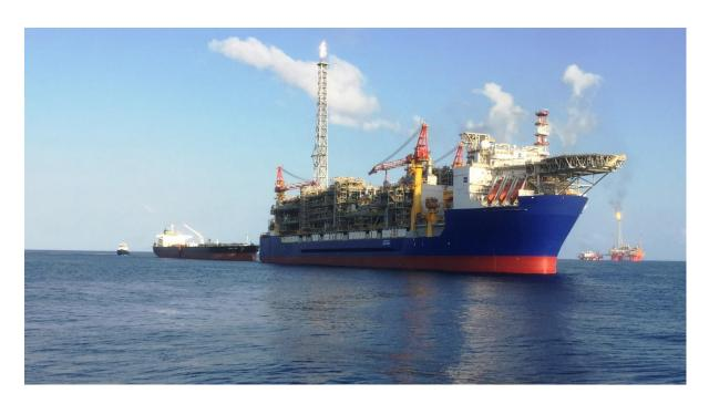
Shipping of condensate from the Floating Production, Storage and Offloading (FPSO) facility "Ichthys Venturer" and the Central Processing Facility "Ichthys Explorer" in the background (far right)
