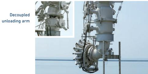
If emergencies including earthquake-triggered tsunami and fires as well as adverse weather and maritime phenomena occur during an LNG unloading operation, the Emergency Release System (ERS) will quickly decouple the arms from vessels without discharging liquid.
