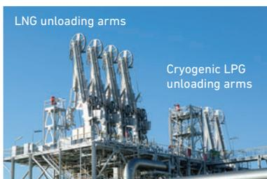
The unloading arms are used to unload LNG/LPG from the LNG/LPG carriers and transfer them to their respective storage tanks. Hydraulic quick couplers installed at the end of the arms ensures safety and accuracy of operations during coupling and decoupling from flanges on the LNG carriers.
