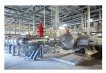
This facility adjusts the calorific value of regasified LNG and natural gas produced in Japan by adding liquefied petroleum gas (LPG). The end product is then transferred to the pipeline network as sales gas.
