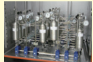
Culture experiment vessels under simulated underground pressure and temperature conditions
