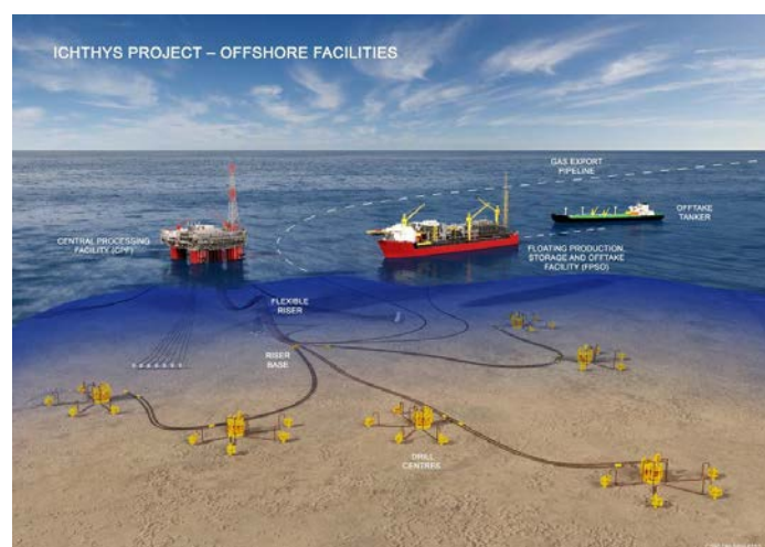
Major Offshore Facilities of the Ichthys LNG Project (Image)
