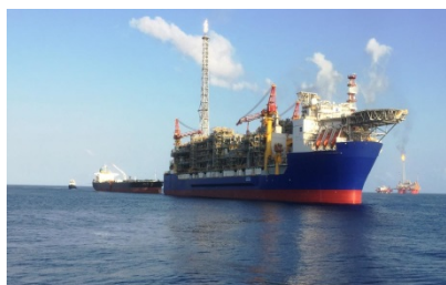
Shipment of condensate from Floating Production Storage and Offloading (FPSO) facility (“Ichthys Venturer”)
