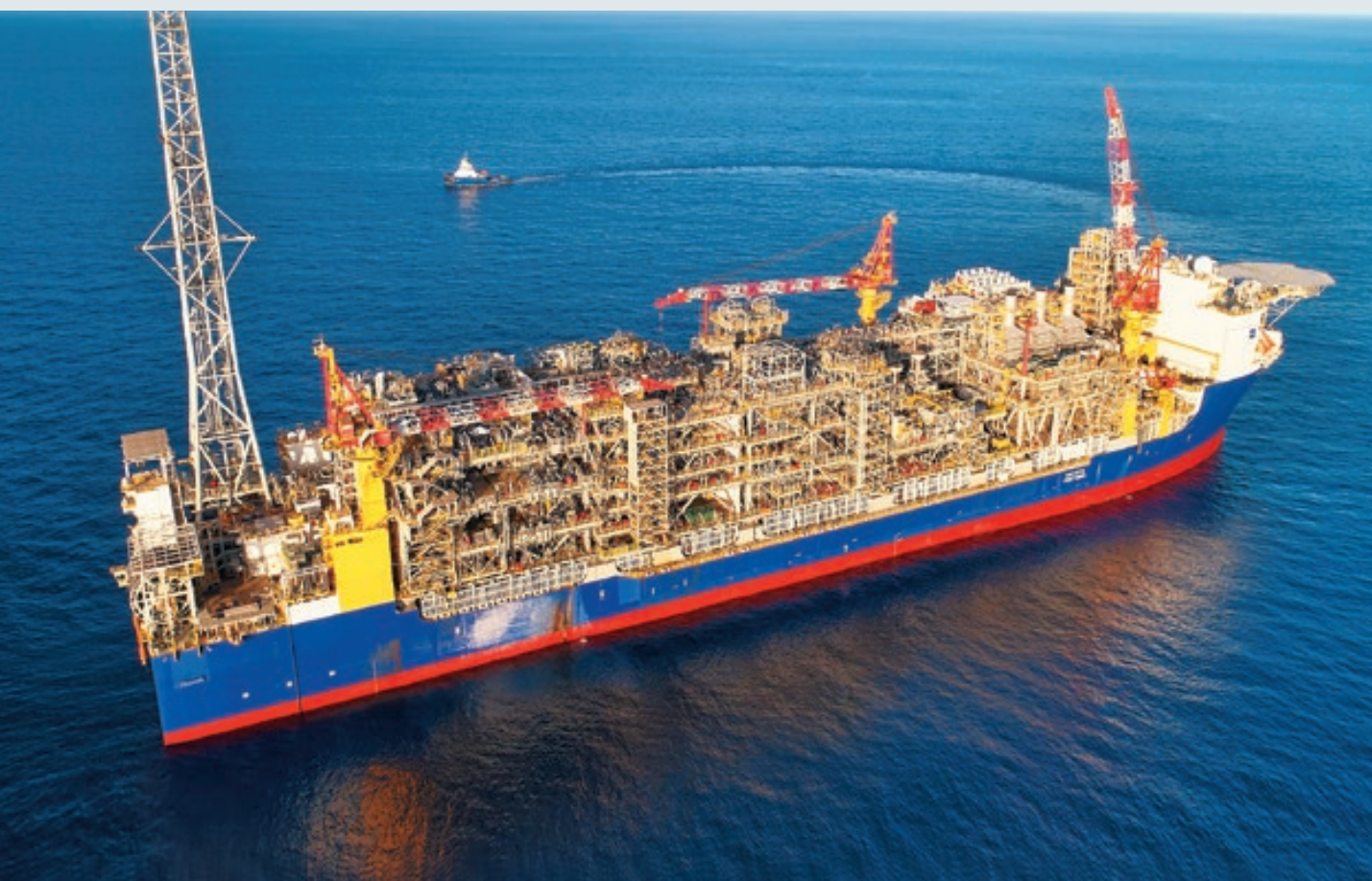
Ichthys LNG Project floating production storage and offloading (FPSO) facility Ichthys Venturer
