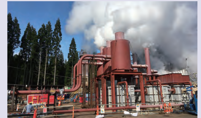
Provisional fumarolic testing of geothermal survey wells in the Oyasu area of Yuzawa City, Akita Prefecture (November 2017)
